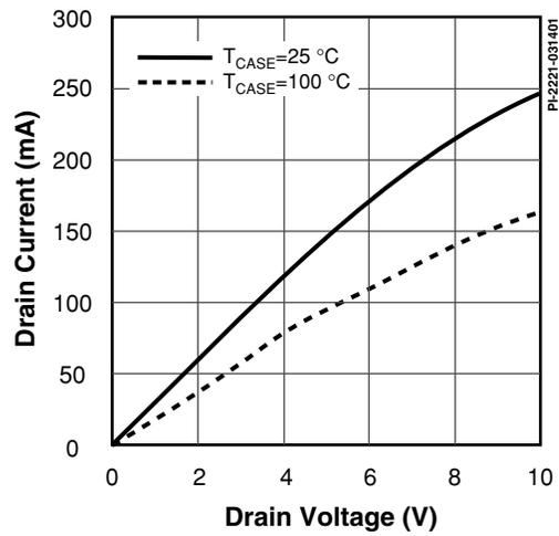
Figure 23. Output Characteristics (DRAIN Current vs. DRAIN Voltage).
