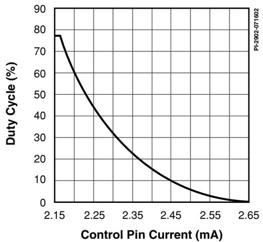
Figure 16. Duty Cycle vs. CONTROL Pin Current.
