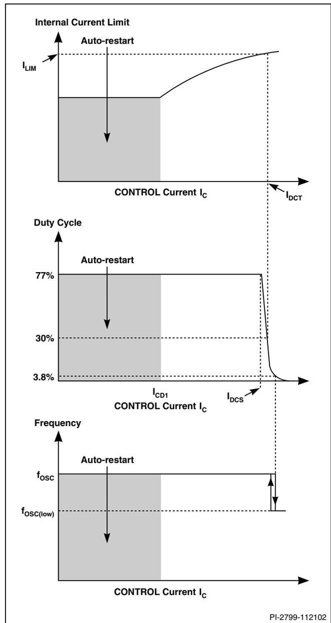
Figure 4. CONTROL Characteristics.
