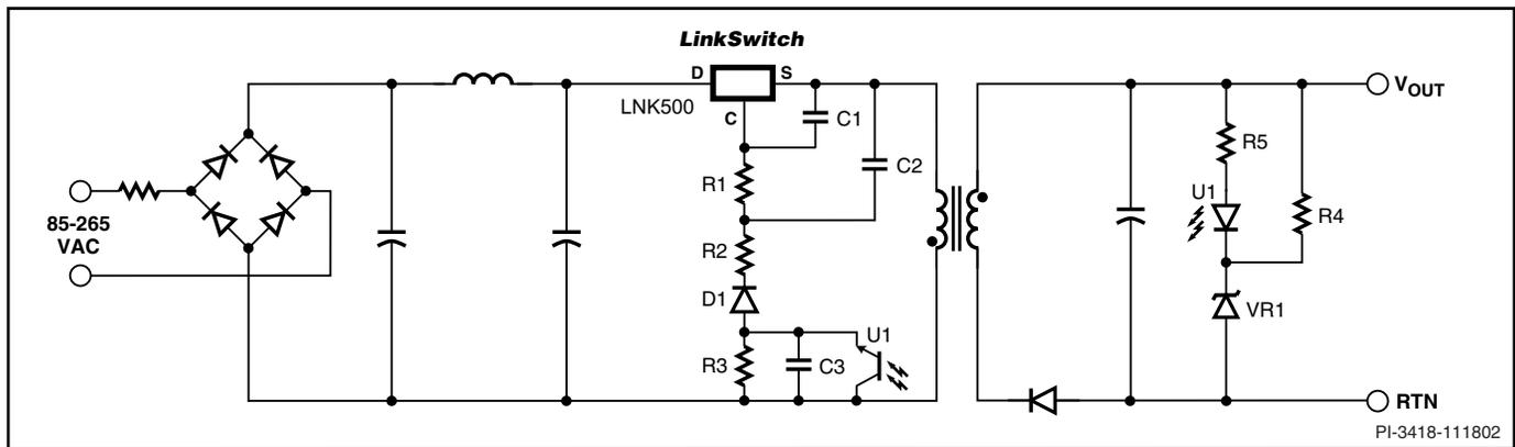
Figure 6. Power Supply Outline Schematic with Optocoupler Feedback.
